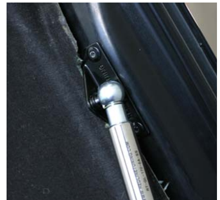
C. Slide clip over ball-stud to lock end-fitting
