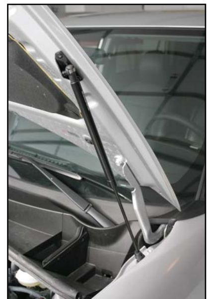
C. Slide clip over ball-stud to lock end-fitting
