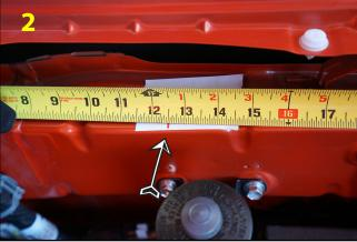
A. Measure and mark 12-1/2" from the front vertical steel behind fender support and put a mark on tape. The bracket will be positioned starting from this line past the 12-1/2" measurement (See Figure 3)
