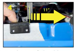
A. Measure and mark 11" from the front vertical steel behind fender support and put a mark on tape as shown. The bracket will be positioned starting from this line past the 11" measurement (See Figure 4 - driver's side view)
