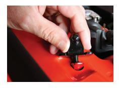
**LEFT** The lower bracket fits neatly in a slotted hole found in every Mustang. Make sure to thread the supplied red attachment nearly all the way down, leaving one to two threads exposed. Then properly align the bracket and slowly finish tightening the bracket in place. The ball stud should point away from the engine.
