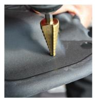
**LEFT** Now remove the battery cover from the car. **RIGHT** Using the punch mark, drill the ¾-inch hole in the battery cover. We used a uni-bit but suggest you use the correctly sized drill bit.
