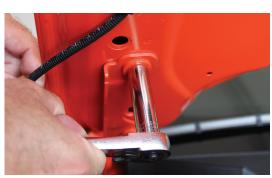
put together, the instructions are clearly written with excellent technical illustrations. Installing the Redline Tuning QuickLift kit is one of the best DIY projects for your new Mustang. You'll need three tools: a 13mm deep socket, a drill with a 3/4-inch or 19mm bit, and a center punch.
