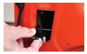
**LEFT** Remove the upper nut on the hood hinge with the 13mm socket, but keep the nut. Repeat on the other side of the engine compartment **RIGHT** Install the hood bracket on each respective side; they are marked "RH" and "LH" for right-hand (passenger) side and left-hand (driver's side). Make sure the bracket is rotated per the instructions, then tighten the nut to secure the bracket.
