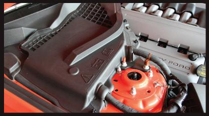
**ABOVE** The battery cover will need to be removed via three push pins and three tabs. Remove the push pin closest to the fender first; the instructions refer to this push pin as "number one."
